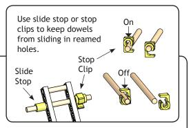
5 Slide stop and a stop clip are put on axles to keep them from sliding out of the reamed holes.
