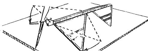
**16**  Pin the wing tips to the cardboard so that the propellor and the rudder touch the board. Now apply extra glue at the joints where arrows point.
