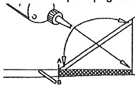
**7**  Cut out the fin, along the edges of the wood, starting at point A around to B.
