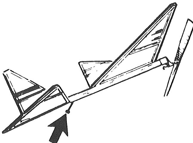
**20**  Tie the rubber motor to make a loop. The loop should be 8-1/2" (216mm) long. Trim the ends to a length of 1/4" (6.4mm). Suspend the rubber band motor from the propeller hook to the slanted pin. Position the knot at the motor hook for smoother running.
