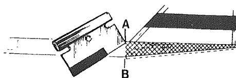
**4**  Apply glue stick to the plan over cross-hatched area. Now, position the balsa wood fuselage (motor stick) on the plan.
