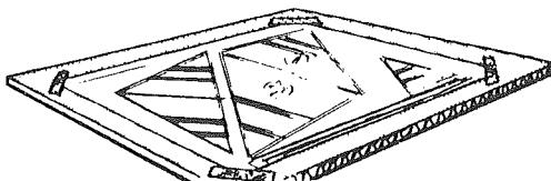
**3**  Carefully slit the plan along the marked line from point A to B.
