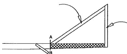
**6**  Apply glue stick to the plan where the wood pieces will fit. Lay wood strips down accordingly. Apply wood glue at the three joints.
