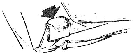
**32**  If, when your model is gliding, it tends to "stall", carefully twist the thin part of the propellor assembly, so that the prop pulls at an angle as shown. Try another test flight. Bend more if additional "stall" correction is needed.
