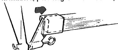
**14**  Glue the wing to the fuselage. Pin in place. The leading (front) edge of the wing should be placed approximately 1-1/4" (31.8mm) from the front edge of the fuselage. DO NOT WAIT FOR THE GLUE TO DRY. DO STEP FIFTEEN IMMEDIATELY BEFORE THE GLUE SETS.
