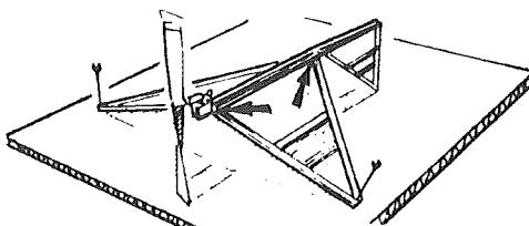
**17**  Glue the horizontal stabilizer (tail) to the rear of the fuselage. Make sure that it is at a 90° angle to the fin.
