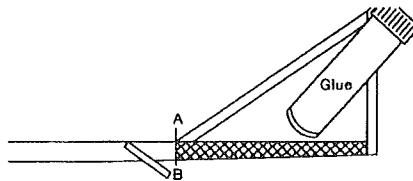
**5**  Carefully cut two of the balsa strips to length to make the triangle fin. Carefully cut the correct angles to form a good fit.
