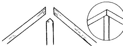
**9**  Frame the wing using the same method as the fin assembly (see steps 5, 6 and 7). Glue each joint securely between pieces as indicated by arrows.
