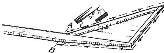
**8**  Cut the wing frame pieces. Be sure to cut them at the correct, precise angles to fit perfectly to each other.
