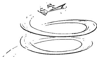
**27**  If your plane flies poorly or makes diving turns into the ground, correct this by installing trim tabs. Trim tab ailerons can be made of stiff typewriter paper measuring 3/4" x 2" (19mm x 51mm) and use a glue stick to apply them as illustrated. If the model tends to drop one wing towards the ground, then bend its tab down 4 degrees at a time. Test fly and adjust as necessary.
