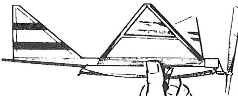
**22**  Wind the rubber band motor clockwise as indicated. Start with 50 turns for short test flights. If it flies correctly increase the turns starting with 100.
