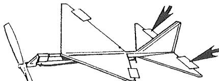
**29**  Finally install one more tab as a rudder on the trailing edge of the fin. Caution: use the rudder as a last resort to correct hard, tight turns.
