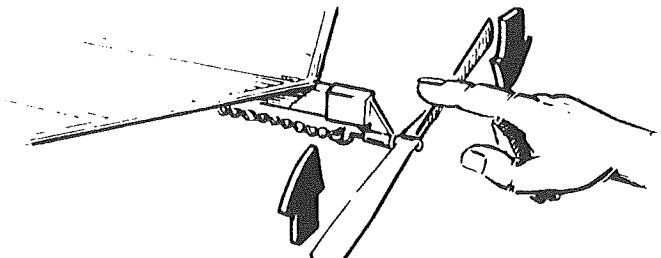
**23**  Hold the propellor. Keep the nose of the Delta Dart in an upward attitude as shown. Release the propellor as you launch the model with a gentle push.
