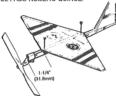
**15**  Turn over the Delta Dart. Hold in place on the cardboard and press the wings down carefully to form the dihedral angle.
