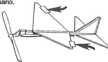
**28**  Next, glue tabs as shown, to the trailing edge of the horizontal stabilizer. Your plane now has elevators. To control a dive, bend them up slightly. To control a stall, bend them down slightly. Test after each slight adjustment.
