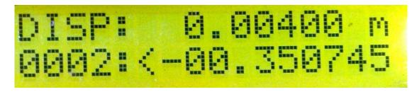
The displacement is displayed in linear vector form considering the start of recording as zero Displacement. With every press of the Memory Review key the reading number is incremented and correspondingly displayed.
