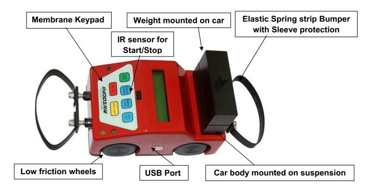
The Car is low friction device and body is mounted on suspension at its wheels. The car has provision for mounting front and rear bumper accessories and weights. It has a 9v replaceable battery and USB port. It has an IR detector for remote timer on/off. The LEDs display the motion status. Duracell 9v battery is recommended.
