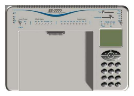
The EB-3000 is a base unit housed in a sturdy plastic case for the electronics and communications experiment plug-in cards.
