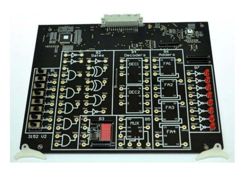
The EB-3152 Multiplexers, Decoders and Adders board is a comprehensive instructional module designed to introduce the student to the basic concepts of various decoders, creating a logic function with a decoder, multiplexers and their use in implementing logic functions and binary arithmetic implementation to students in high schools, technical schools and colleges.
