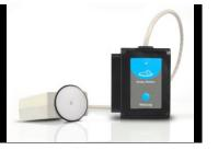
Your rotary motion sensor needs to be connected to a WIFI-201 module. The WIFI-201 module will create a closed NeuLog wifi network which will stream the NeuLog data to a device of your choosing. Once your device is wirelessly connected to the NeuLog network you can run experiments and collect data through a browser of your choosing.
