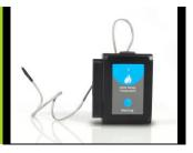
Because the metal wires have different properties both heat and electricity are conducted at different rates. Using the Seebeck Effect, a voltage is created in the wires. Different voltages are produced at different temperatures. The voltage is what is directly measured and then translated into a very accurate temperature reading.
