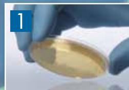
Gently press plate to surface to collect sample.
