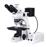
nator includes adjustable field and aperture diaphragms to minimize reflections and optimize performance. Conversion of the standard halogen illumination to a 3W LED is easily achieved with a simple plug-in module.
