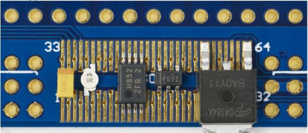
**Figure 2)** Starting from left to right, a surface mount Buck Regulator IC in a 8-SOIC package, fits well skipping over pins on the board. The next part is a Schottky diode in a SOD-123 package. This part spans the open area and fits well on the boards SMD pins. The last part is a FTDI FT232RL IC in a 28-SSOP package. It matches up to each pad, pin for pin.
