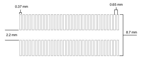
Compatible device packages include, but not limited to SO type, 0603, 0805, SOT-223, CDFP and SSOP components. Below are just a few examples of how the Propeller Project Board's SMD pads that can be used in your projects.
