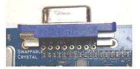
Once the VGA connector is in place, you will have access to vertical and horizontal synchronization, as well as red, green and blue. The only thing you need to do is connect the I/O pins you're going to use. The support circuitry is built into the board (see schematic for details).
