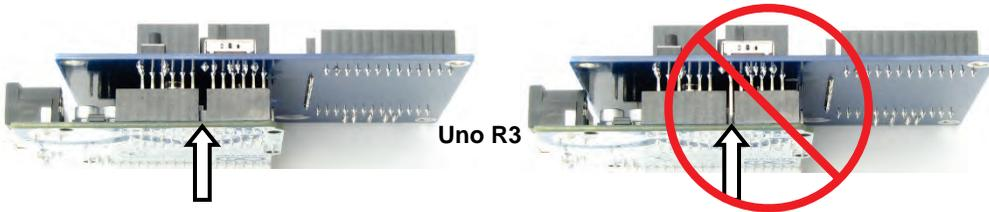
*Correct: gap in pins lines up with gap in sockets.*
