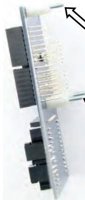
*Slide Nylon spacers over screws. A spacer may not fit with the screw that goes by the Arduino Uno's reset button.*
