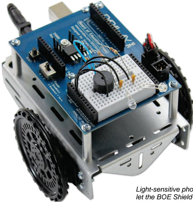
*Light-sensitive phototransistors let the BOE Shield-Bot navigate by driving towards a bright light source.*
