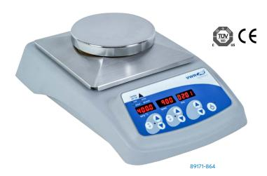
**Heat caution indicator:** For additional safety, a hot-symbol warning light is illuminated when heat is turned on and remains on until top plate cools down.
