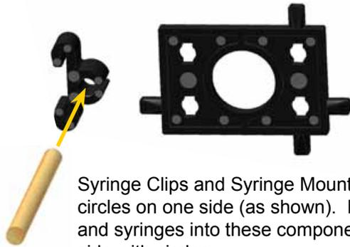
Syringe Clips and Syringe Mounts have circles on one side (as shown). Insert dowels and syringes into these components from the side with circles.
