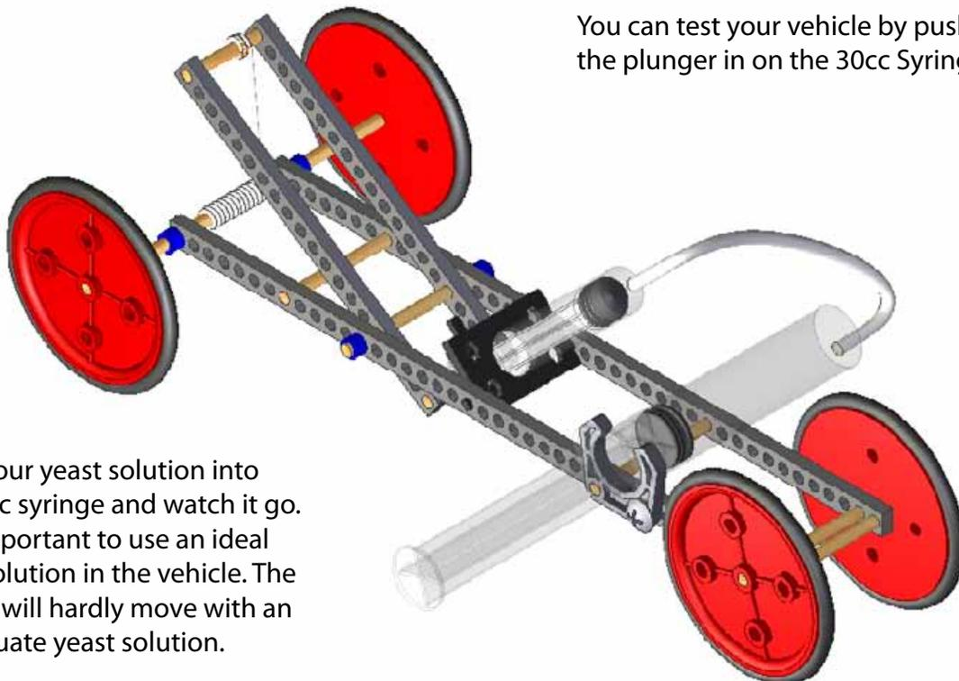
Place your yeast solution into the 30cc syringe and watch it go. \*It is important to use an ideal yeast solution in the vehicle. The vehicle will hardly move with an inadequate yeast solution.
