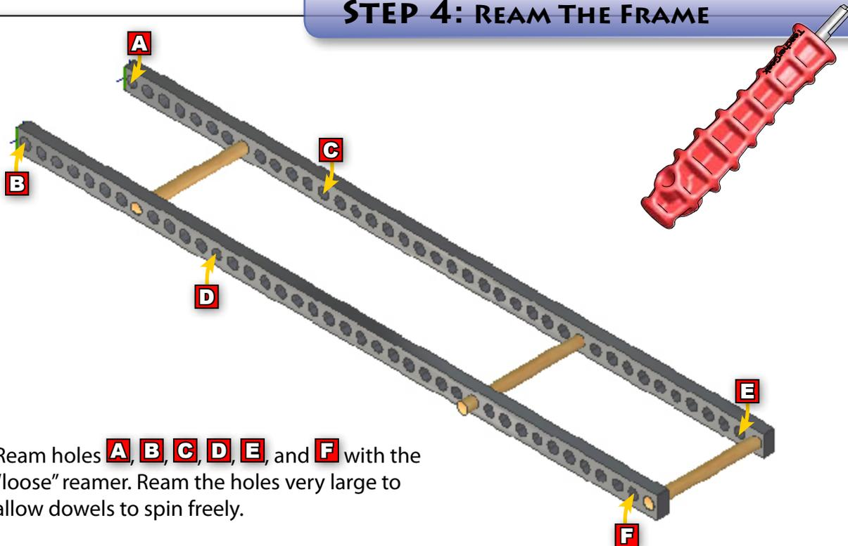
Ream holes **A**, **B**, **C**, **D**, **E**, and **F** with the "loose" reamer. Ream the holes very large to allow dowels to spin freely.
