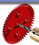
Pull and push the reamer in and out of the hole.
