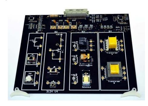
The EB-3124 Magnetism and Induction board is a comprehensive instructional module designed to teach the fundamental concepts of magnetism, electromagnets and transformers to students in high schools, technical schools and colleges.
