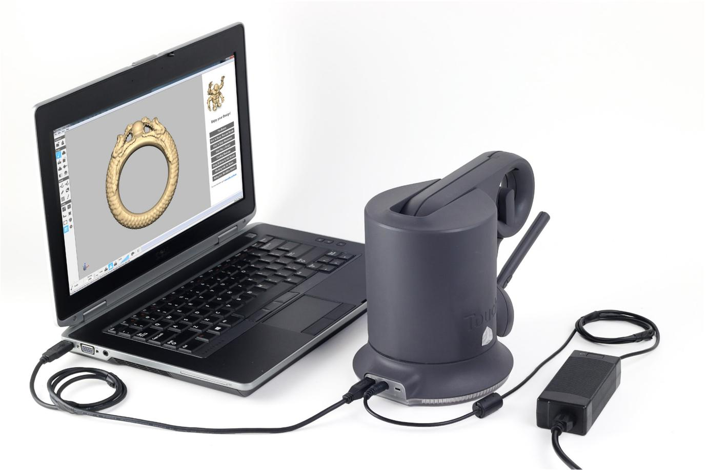
7. Make sure that the **LEDs ring** at the base is lit **Blue**. Blue indicates the Touch has power. If it is not, check all of the connections. If the problem continues, contact 3D Systems customer support.
