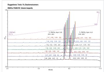
**Figure 6.** Here, a 150mm-long DNAPac PA200 RS column was run for >350 gradient cycles with injection of different sets of ONs each 20 cycles. The gradient was 350–675mm NaCl in six column volumes at pH 8 and 30°C at a linear velocity of 1.12mm/sec. At this flow the maximum pressure was 5800psi (400 bar).
