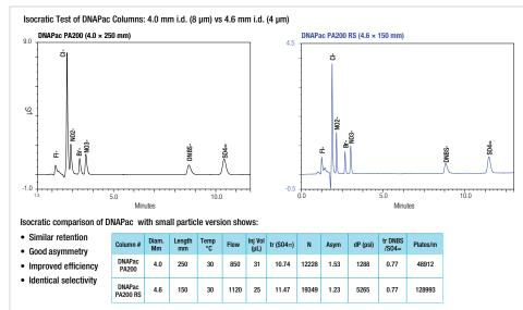
**Figure 1.** Isocratic elution of seven small anions employed 1.7mM NaHCO<sub>3</sub> and 1.8mm Na<sub>2</sub>CO<sub>3</sub> at a linear velocity of 1.12mm/s using a Dionex ASRS-300 to suppress background signal.
