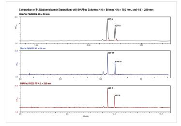
**Figure 5.** A 21-base ON (eGFP-S) was chromatographed on the DNAPac PA200 RS in three lengths: 50, 150 and 250mm. In each case the diastereoisomers are readily resolved from one another. The 250mm column completed the separation in ~10.5 min, the 150mm column resolved the isomers within 7.5 min, and the 50mm column completed the separation in 2.6 min. These separations are difficult with other chromatographic modes. Conditions are the same as in Figure 4 for RS column.
