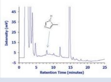
Figure 2: Chromatogram showing retention of 4-MI (300  $\mu$ g/mL standard solution) on a 100x2.1mm id Purospher\*STAR RP-18e column.
